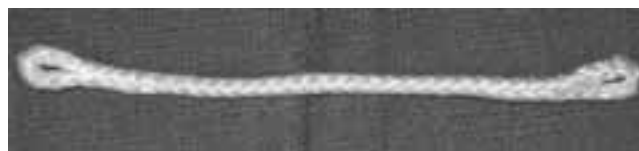
Figure 1. The ultra-high molecular weight polyethylene (UHMWPE) braided graft manufactured by Smith & Nephew Richards, Inc. (Memphis, TN)
