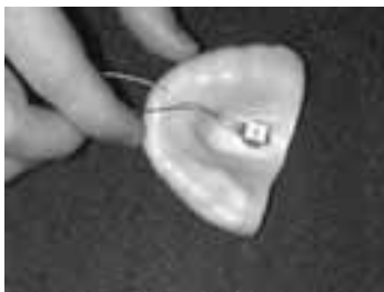
Figure 3. Custom-made mouthpiece with tri-axial accelerometer.
